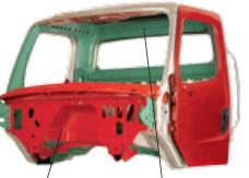
**Aluminum Structural Reinforcements** E-coated Steel Reinforcements
