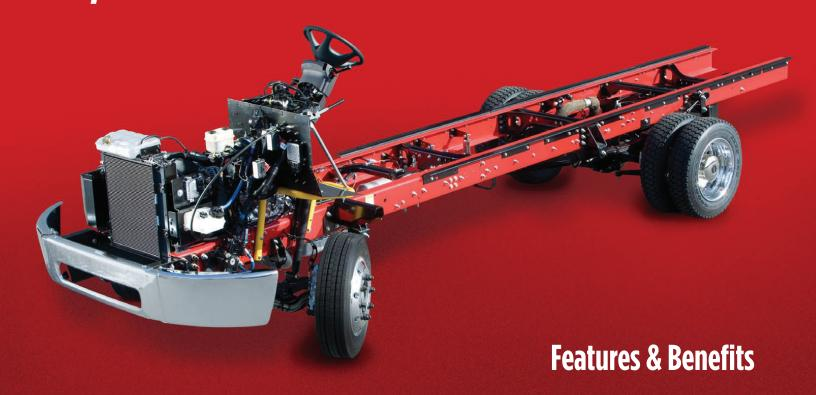
As part of our pledge to help you consistently deliver more profit, we are proud to introduce a gasoline-powered chassis to our WIV product lineup, available on either the MT-45 or MT-55 chassis models. Offering a gross vehicle weight rating of up to 23,000 lb. and 308 horsepower, the new gas WIV chassis from FCCC is a powerful new performer, ready to take on large cargo and heavy-duty loads.
